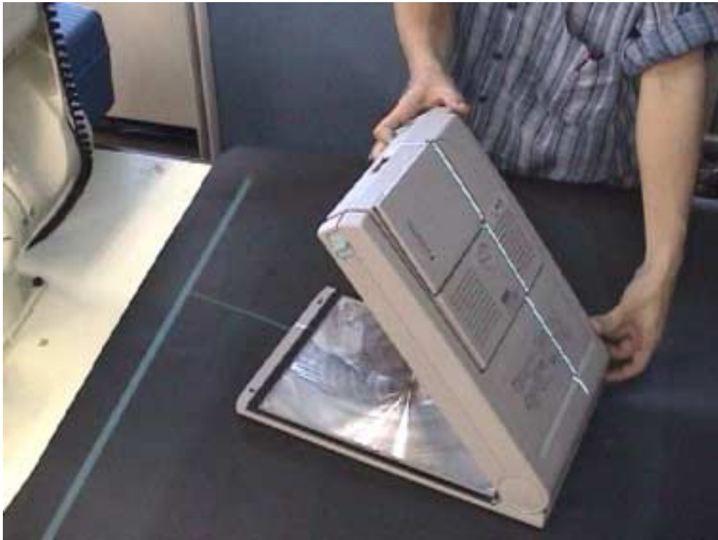
☒ 4.26: A striped light is projected to check the height of the main body.
