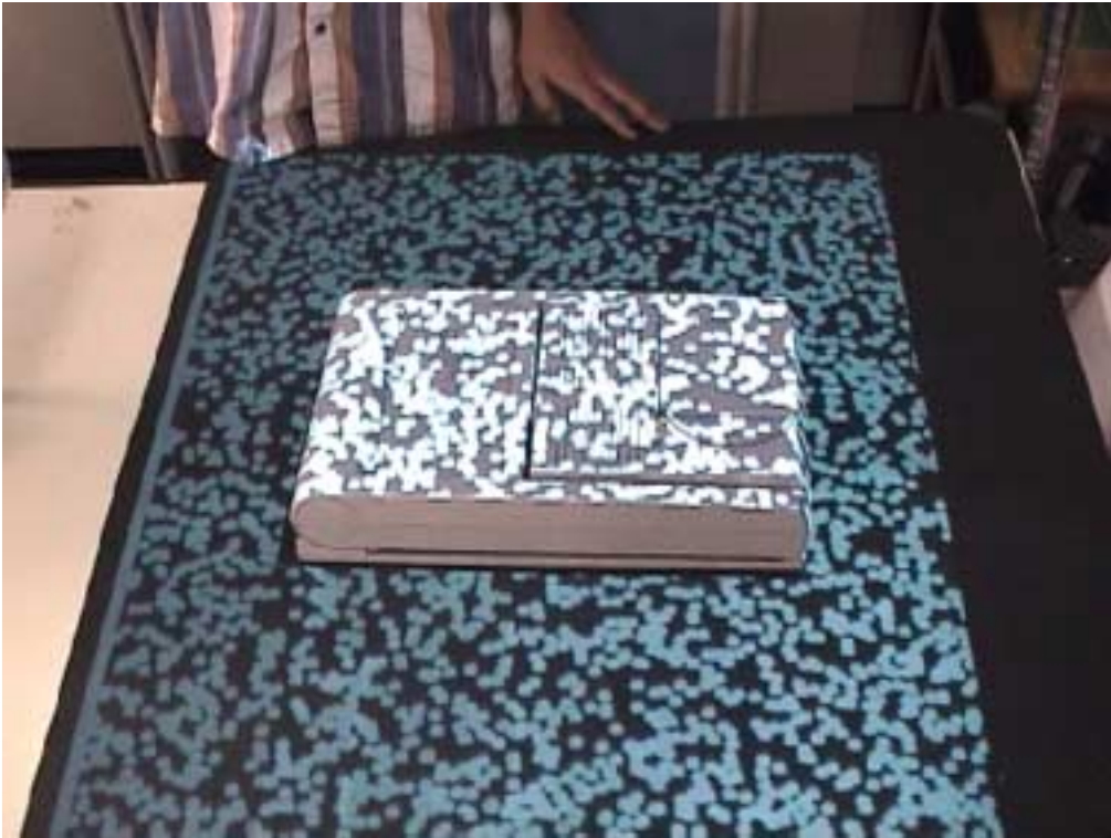
图 4.17: A scene of 3D measurement using the random-dot stereo
