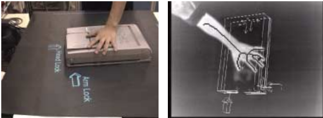
図 4.21: An infrared image for detecting the human hand. The thinning results and the object model are superimposed.
