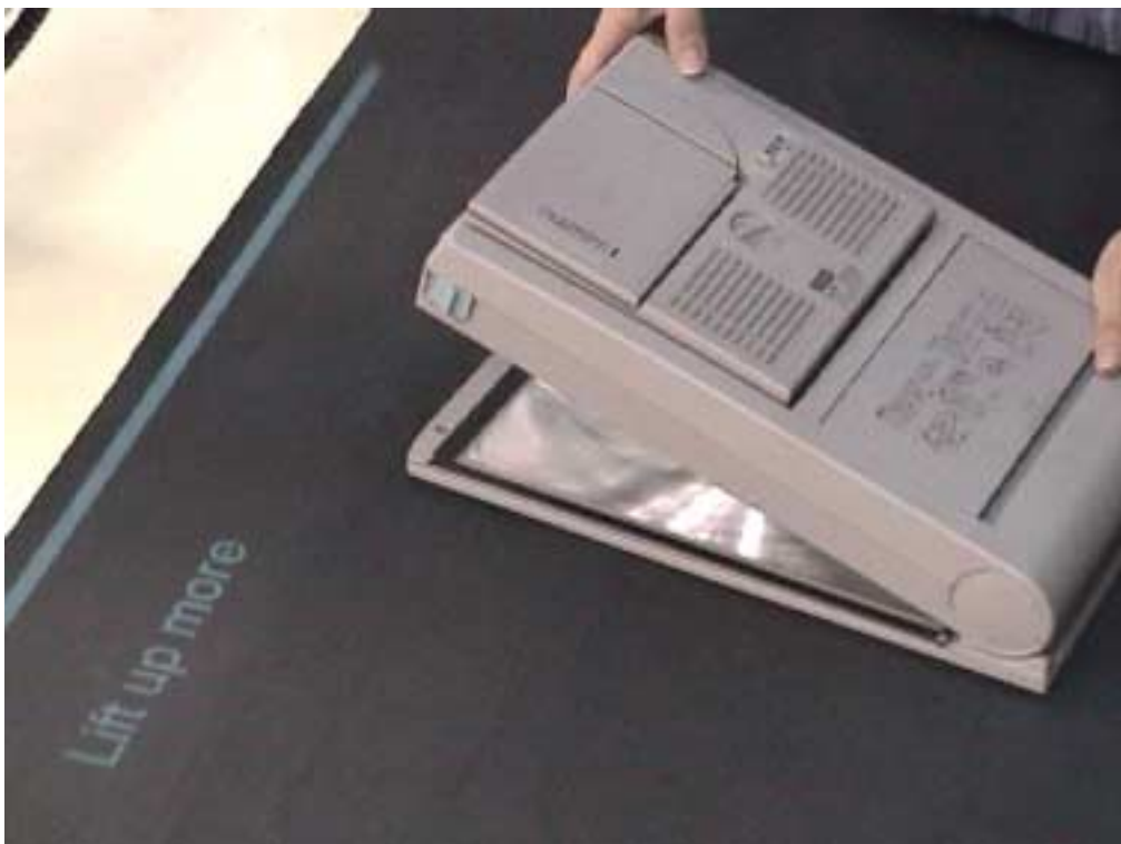
☒ 4.27: The message, "Lift up more" is projected when the height of the main body is smaller than model.
