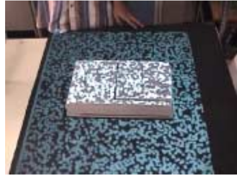
Figure 4: A scene of 3D measurement using the random-dot stereo
