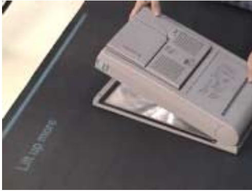
Figure 11: The message, “Lift up more” is projected when the height of the main body is smaller than the model.
