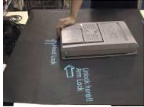
Figure 9: Adaptive annotation by monitoring the user's action
