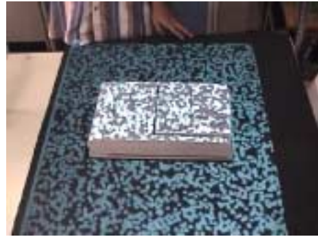
Fig.4: A scene of 3D measurement using the random-dot stereo
