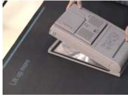
Fig.11: The message, "Lift up more" is projected when the height of the main body is smaller than the model.
